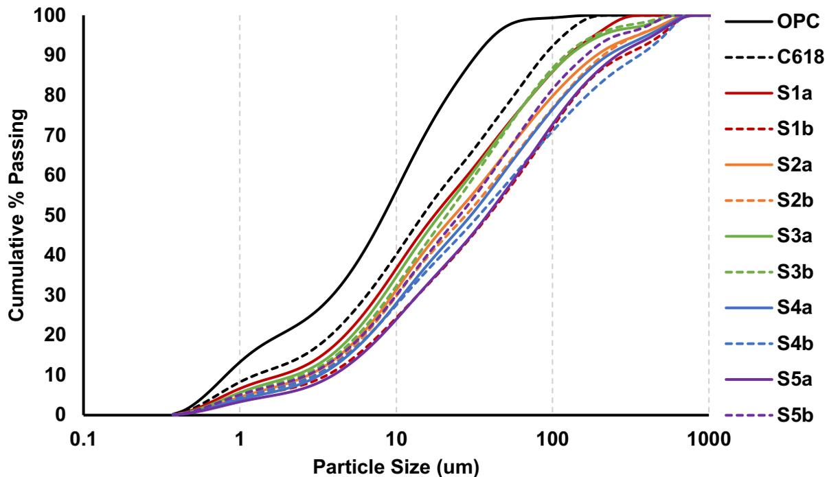
**Figure 1** - Cumulative percentage of fly ash particles smaller than a given size for the fly ash samples, a typical OPC, and an ASTM C618 Class F fly ash.
