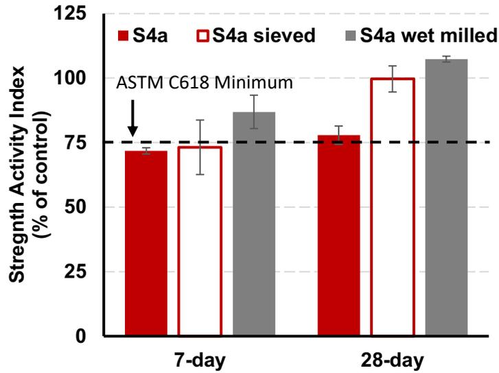
Figure 11 - SAI of as-received, sieved, and wet-milled S4a fly ash.
