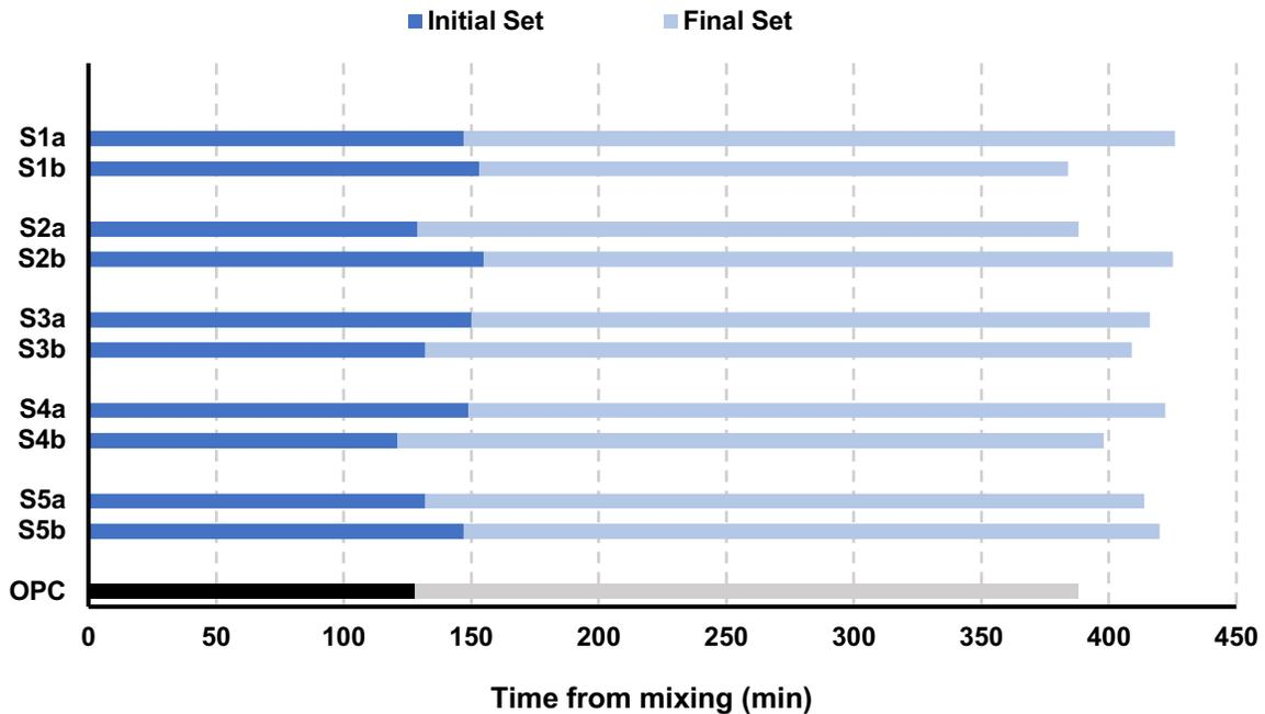
Figure 7 - Effect of fly ash on mortar initial and final setting times.
