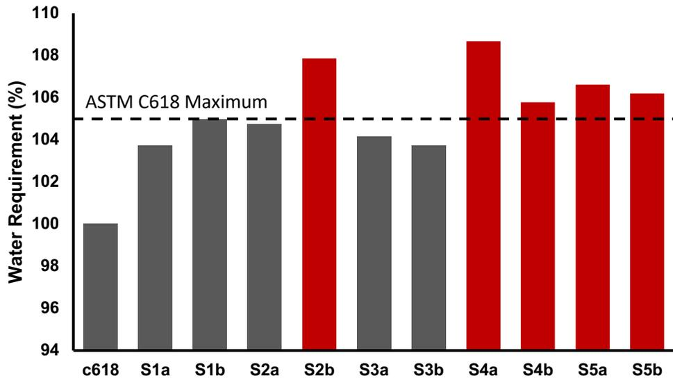
**Figure 4** - Water requirement, or the relative effect of the ash samples on flow of a fly ash-cement mortar compared to the OPC mortar. ASTM C618 allows a maximum water requirement of 105% of the control.
