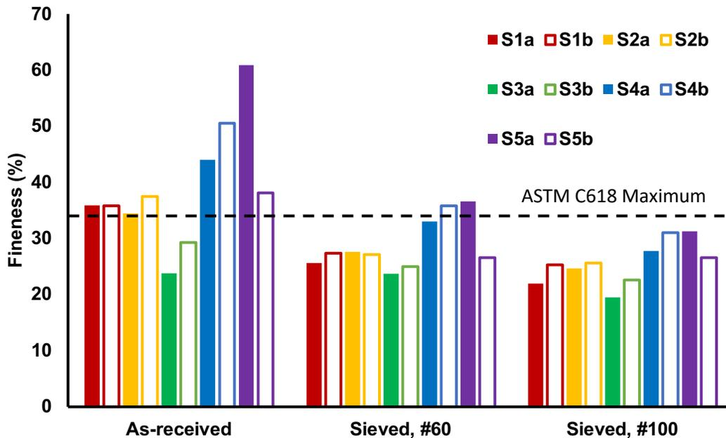
**Figure 3** - Fineness of the fly ash samples before and following sieving. ASTM C618 allows a maximum fineness of 34%. This value corresponds to the proportion of the mass of material in a sample greater than 45  $\mu\text{m}$  in diameter.
