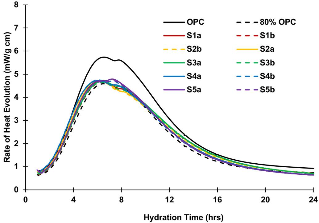
Figure 6 - Hydration kinetics of 100% OPC or 80% OPC + 20% fly ash pastes at a w/c of 0.40.
