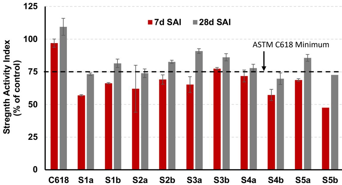
Figure 9 - Strength activity indices of the fly ash mortars at 7 and 28 days.
