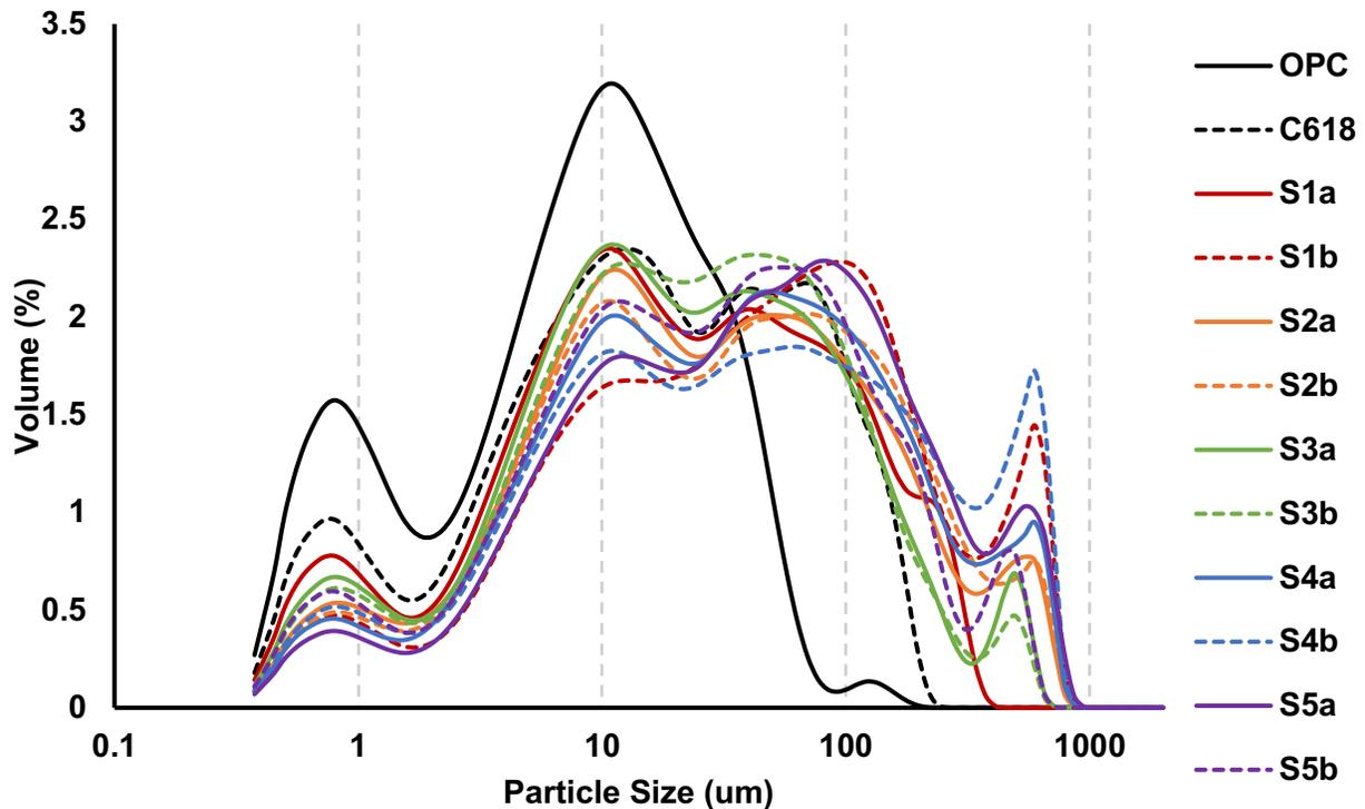
**Figure 2** - Distribution of particles sizes for each of the fly ash samples, a typical OPC, and an ASTM C618 Class F fly ash.
