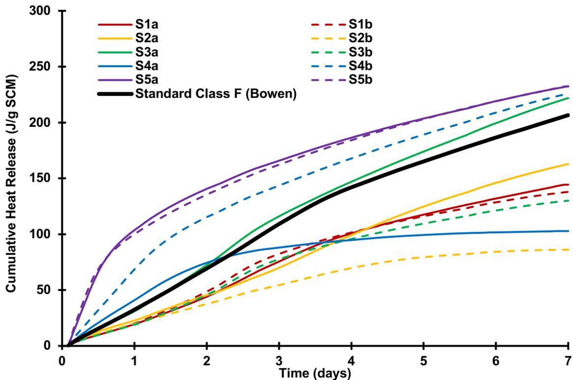
**Figure 8** - R<sup>3</sup> calorimetric testing of fly ash pozzolanic reactivity.
