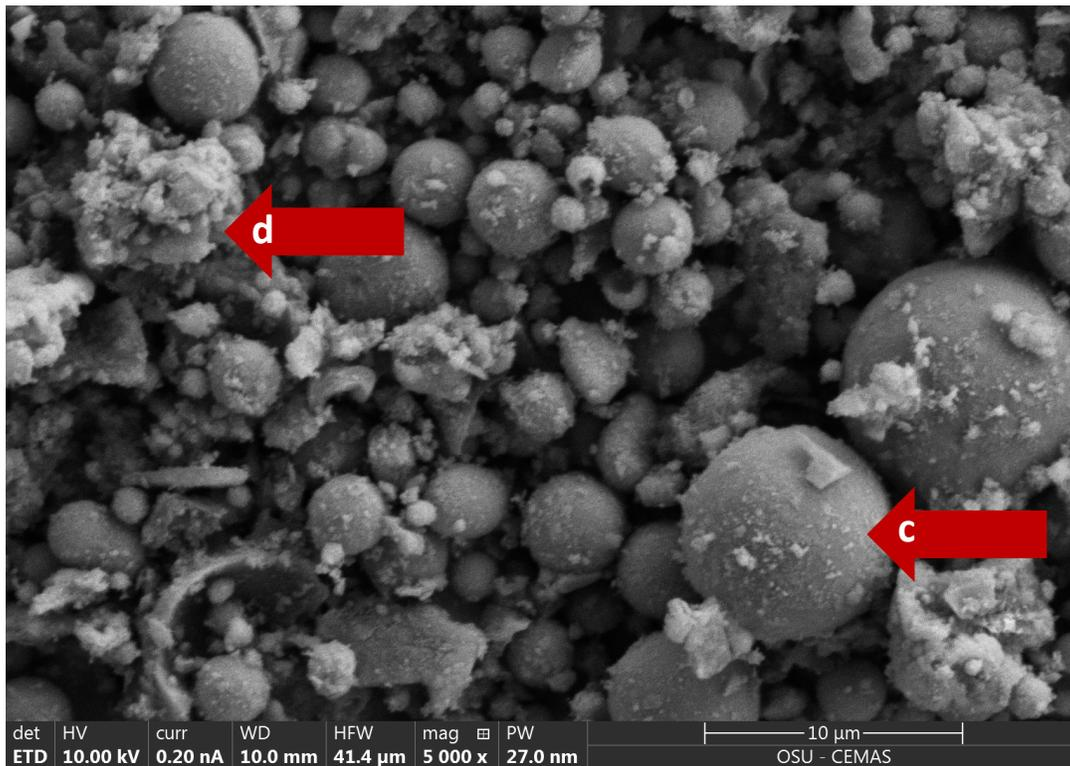
**Figure 5** - SEM images of sample S4a showing the presence of non-spherical particles, and possible hydrated components, both independent of the fly ash particles and on the surface of the fly ash.
