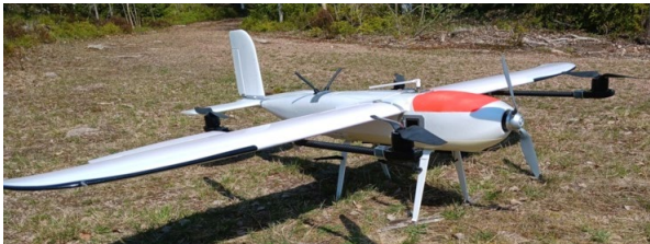
Figure 1. Loong 2160 drone with the antennas placed on the front top, rear bottom and legs of the landing gear.
