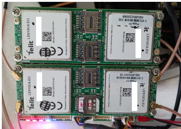
Figure 2. Elsie's Halo OEM Platform supporting four simultaneous LTE connections
