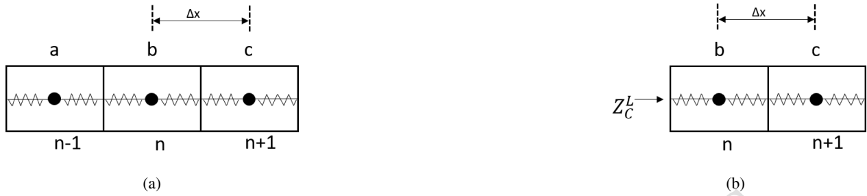
Figure 2: Discretized CAFE domain: (a) a standard arrangement of three cells, (b) analogous setup where the left cell is replaced by an impedance.
