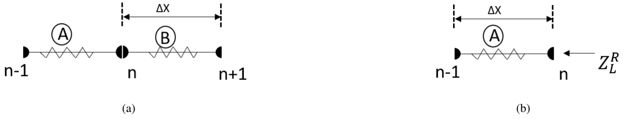
Figure 1: Discretized LISA domain: (a) a standard arrangement of two cells, (b) analogous setup where the right cell is replaced by an impedance.
